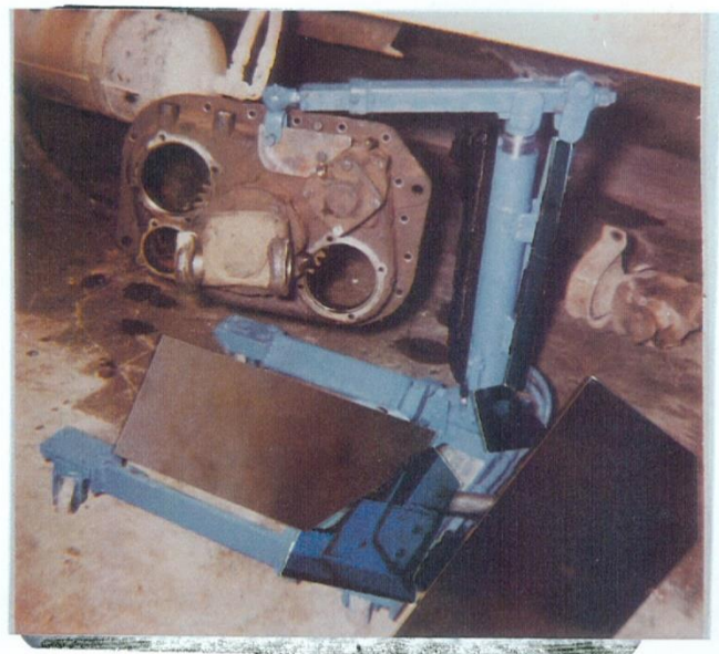
SPLITTER BOX AFTER REMOVAL, IS TRANSFERRED TO THE SHOP
